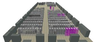
6SigmaAccess is a browser-based tool that reduces the capacity planning process from weeks to hours by consolidating critical data center resources in a singular view. Backed by our advanced CFD software, 6SigmaRoom, 6SigmaAccess enables you to accommodate future capacity planning requirements by predicting the impact of any change within your facility.
